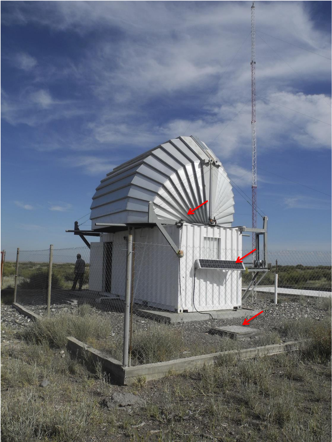
Figure 4. Las Amarillas station (LAMA). Arrows show GPS, solar panel and sensor vault.
